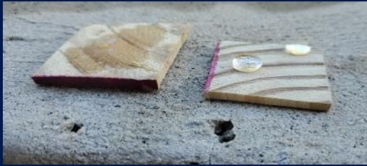
Wood: Left = Uncoated. Right = Coated with Pipedream Additive
