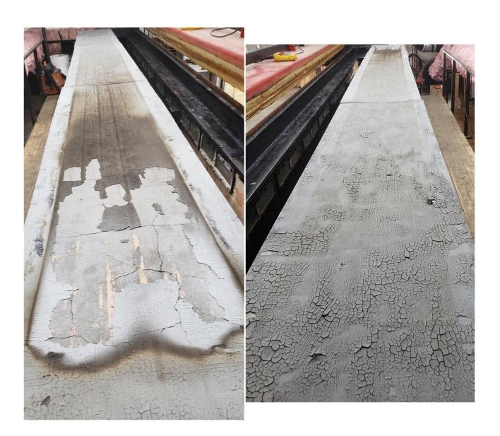
**Photograph No. 2:** The 24-foot long test speicimen after being subjected to the 10-minute flame exposure from the test chamber's burner end (left), and the vent end (right).
