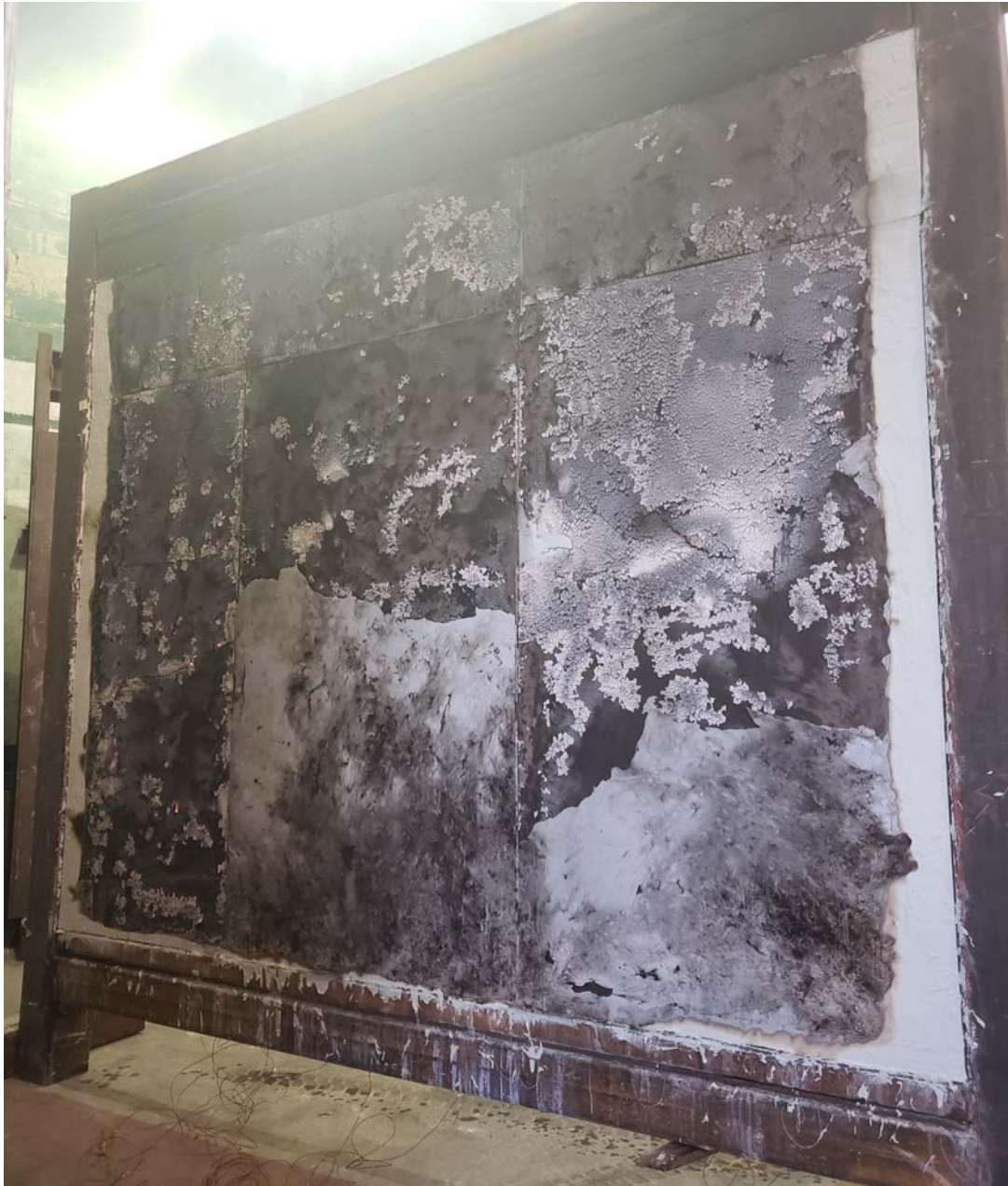
Figure 8: The exposed face of wall assembly after the test
