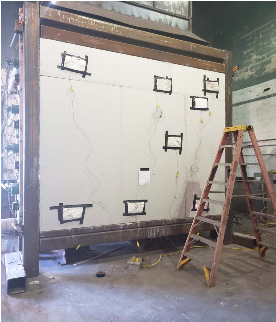
Figure 7: The unexposed face of wall assembly prior to testing.
