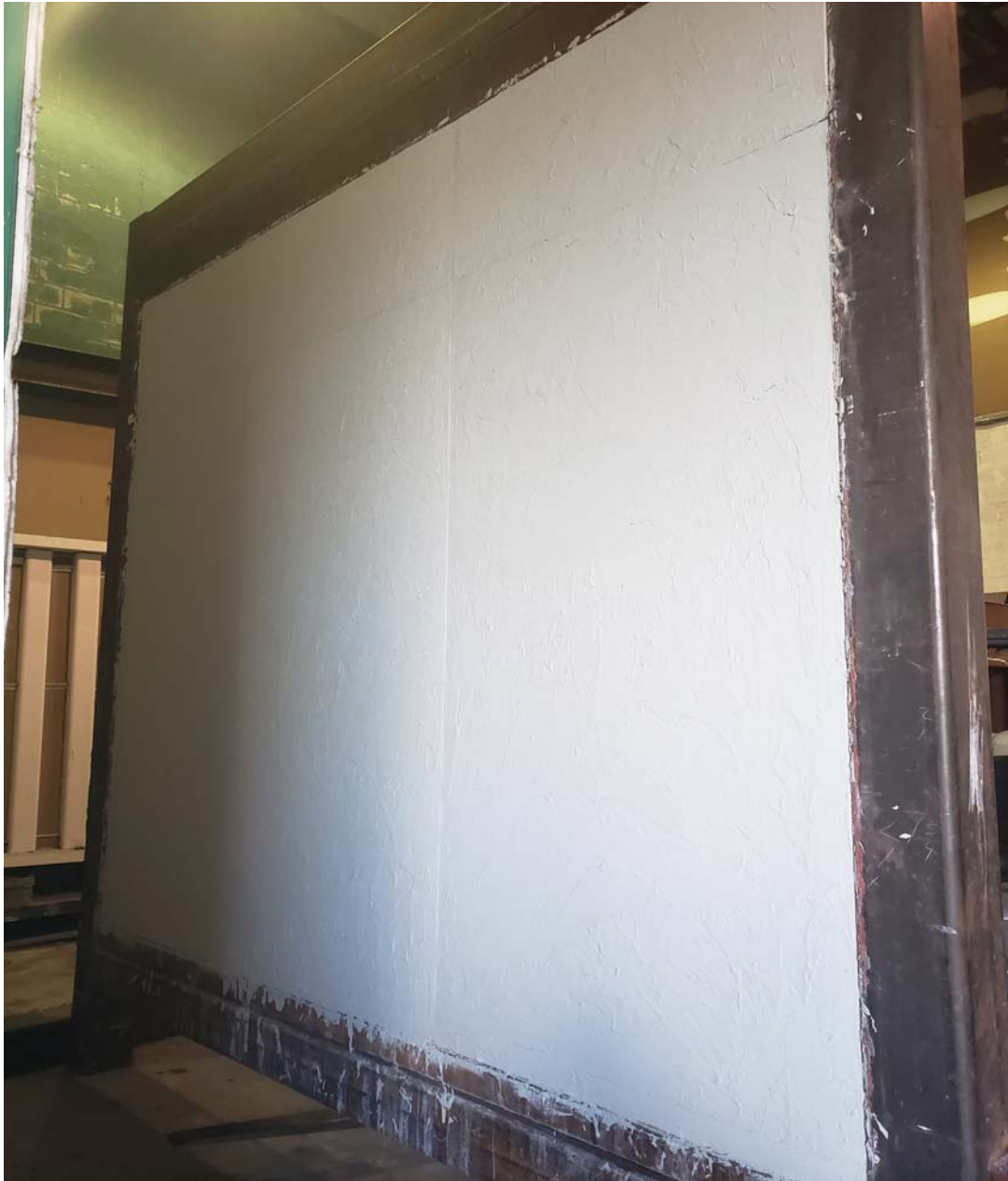
Figure 6: The exposed face of wall assembly prior to testing.
